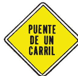
One Lane Bridge
