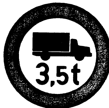
Fig 13a—Traffic Prohibited for Trucks Above a Specified Authorized Total Weight
