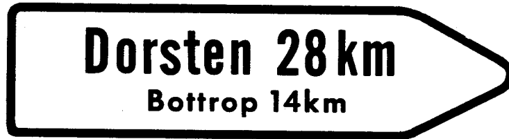
Fig 42-- Direction Sign for Other Permanent Roads
