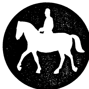
Fig 17a—Authorized for Riders (Use of the indicated path or section of the road prohibited for all other traffic participants)
