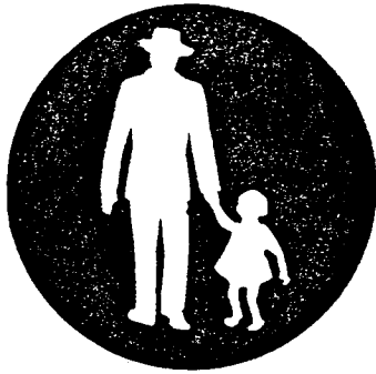
Fig 17b—Authorized for Pedestrians (Use of the indicated path or section of the road prohibited for all other traffic participants)
